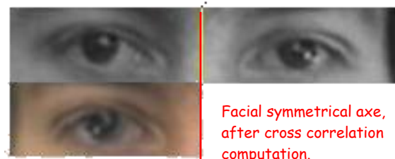
Superposition of the two pictures (Maximum of the cross correlation function)
