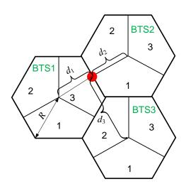
Then calculate the transmission losses:  $L_{p1}(d)$ ,  $L_{p2}(d)$  and  $L_{p3}(d)$ , SIR and throughput.
