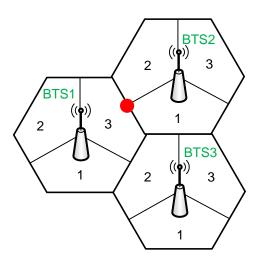
We assume the radius of the cell:  $R = 500\,m$ . The quality of the received signal for the MS from the serving cell in different system configurations needs to be determined. All BTSs transmit with the same power. The sectors are the same, divided into 120°. The radiation pattern of the antenna system is as follows:
