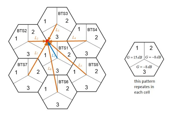
Based on the above picture loss for the desired signal from sector 1  $L^a_1$  can be calculated, as well as losses of the interfering signals from cells 2,3,4,5,6,7:  $L^a_{2,3,4,5,6,7}$
