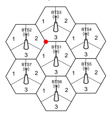
, which consists of seven cells with a radius of:  $R=1~\mathrm{km}$ . We are interested in the quality of the received signal at a specific UE location (marked with a red circle), which it receives from each BTS in different configurations.
